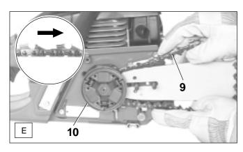
Lift the chain (E/9) over the clutch drum and onto the sprocket (E/10). Using your right hand, guide the chain into the top guide groove on the guide bar (D/8). Note that the cutting edges along the top of the chain must point in the direction of the arrow!
